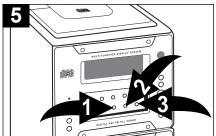
Press the TUNING/CD SKIP/ SEARCH (►►) ① or (►<) ② button to set the current minute. Press the MEMORY/TIME SET button ③ and the time will be set.
